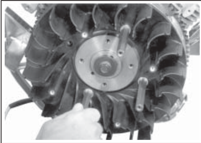
Figure 11-28. Installing Supports for Metal Grass Screen.
